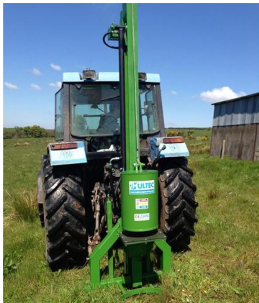
Plate 4: Tractor mounted auger type post hole digger
